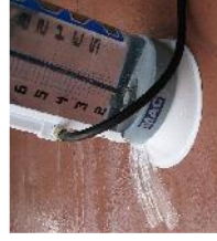
Lean to Drain Rest to drain the chamber
