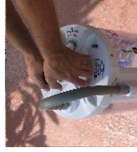
Ease tension while leveling by squeezing shaft knob downward with the aid of the handles
